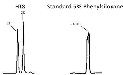
Chromatogram on the left clearly demonstrates the significant difference in selectivity of the HT8 column. By GC/MS, quantitation of CB28 using a standard 5% phenylpolysiloxane column is impossible as coelution with CB31 (with the same number of chlorines) occurs.
