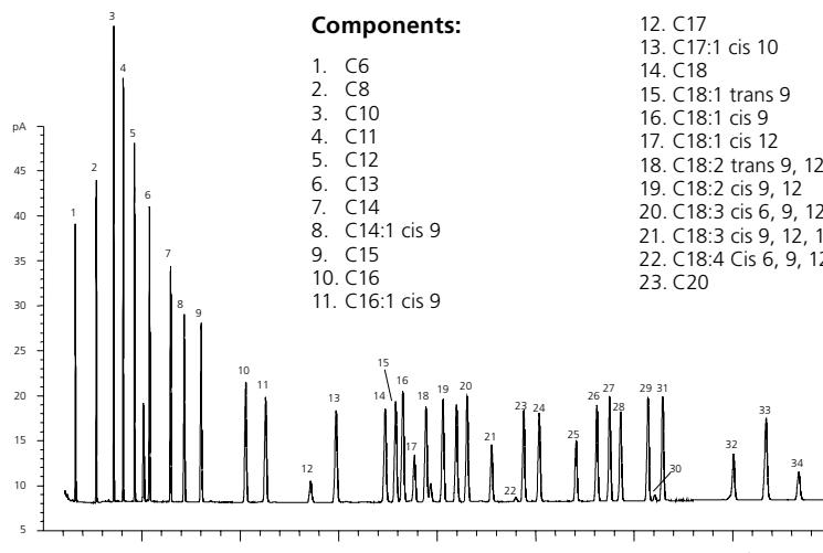
Notes: The chromatogram shows the excellent separation of a complex mixture of FAME compounds. Note the excellent peak shape and separation of the Omega-1,2 and 3 fatty acid isomers both structural and cis and trans.
