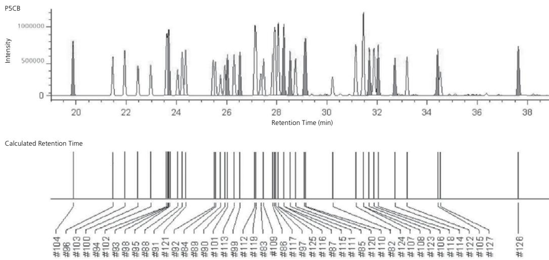
The separation of a mixture of pentachlorobiphenyls using an HT8-PCB column. Elution order calculated for the 5CBs from structure activity relationships based on coplanarity and confirmation, steric factors and electron density show a high correlation with experimental results.
