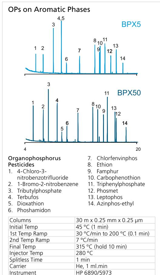
Effect of increasing Phenyl content in the stationary phase.
