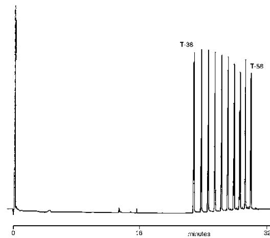
Notes: For the analysis of triglycerides, on-column injection is recommended. Temperatures above 380 °C are not recommended as triglycerides can degrade.
