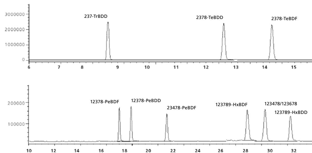
Figure 4. The separation of a mixture of PBDD and PBDF on a BPX70 column. The mixture was separated using the  $\pi-\pi$  interaction between the compounds and the cyano phase of the BPX70 column.
