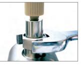
Install entire assembly into pump head.
