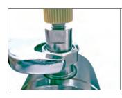
Place wrench on the hex nut and turn. The hex nut or thread ring will turn independently of the fitting connection.
