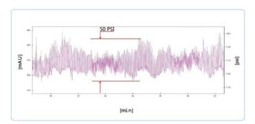
L-3245 is able to stably deliver mobile phase even under 7000PSI. (Figure right)
