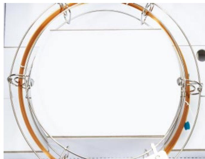
Secure-Lock™: Column in release-position
