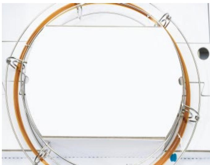
Secure-Lock™: Column in locked-position
