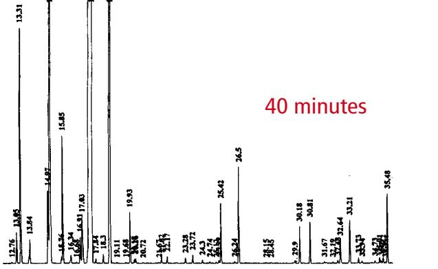
**Fig. 9. Lemon oil in a 100 µm column**
