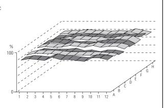
Note the high recovery (y axis) with an average deviation across the 96 wells of just 3.2% (well positions are shown on the x and z axes). SPEC provides the predictable flow characteristics analysts require for true walk-away automated processing. With SPEC you need not worry about clogging, and as an added benefit, the typically low vacuum pressure requirement prevents cross-talk (e.g. spraying of fast running eluates between wells in the collection plate).
