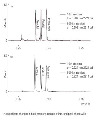
Captiva ND<sup>Lipids</sup> after 10 and 5010 injections for LC/MS or LC/MS/MS bioanalysis (top = UV detection; bottom = MS detection).
