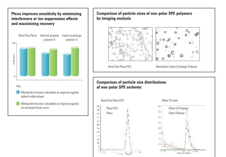
The narrow particle size distribution offers reproducible, superior flow characteristics with minimal clogging
