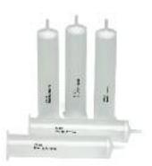
Empty SPE cartridges with two frits (pre-inserted), 60 mL, 12131018
